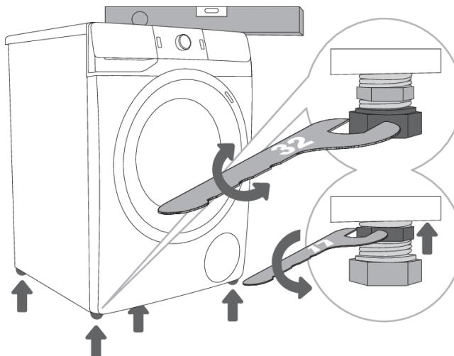
**1** Level the washing machine in longitudinal and traverse direction by rotating the adjustable feet.
