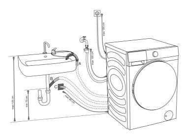
A Discharge hose end may be placed over a sink or a bathtub. B Use a string fed through the opening in the elbow support to attach the hose and prevent it from slipping to the floor.
