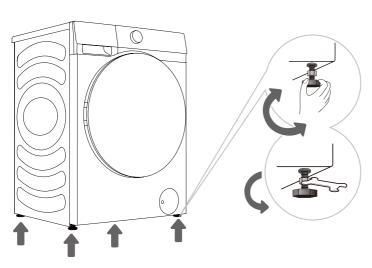
**1** Rotate the adjustable feet to level the washing machine lengthwise and crosswise. The feet allow levelling by +/- 2 cm.
