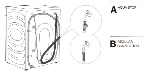
$\frac{1}{9}$  For normal washing machine operation, the pressure in the water mains should be between 0.1–1 MPa (1-10 bar; 1–10 kp/cm<sup>2</sup>; 10–100 N/cm<sup>2</sup>). Minimum dynamic water pressure can be determined by measuring the water flow. In 15 seconds, 3 litres of water should flow from a fully open tap.
