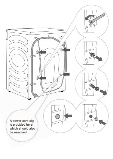
**1** Move aside the hoses and use a fitting spanner to undo the 4 screws on the back of the appliance by turning them counter clockwise, as indicated by the arrow. Undo them by approximately 30 mm (not completely).
