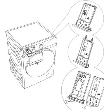
1. Open the detergent compartment, press the limit lever as shown in the figure, and pull out the detergent compartment;
