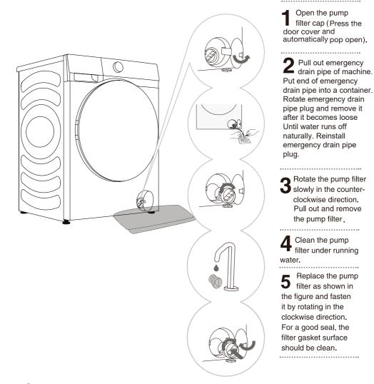
'ở The pump filter must be timely cleaned, especially after washing very fleecy, woolly, or very old laundry.
