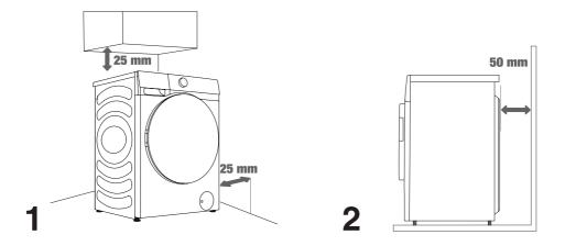
$\dot{\phi}$  The washing machine may not be in contact with a wall or adjacent furniture. For optimum washing machine operation, we recommend observing the clearances from the walls as indicated in the figure.
