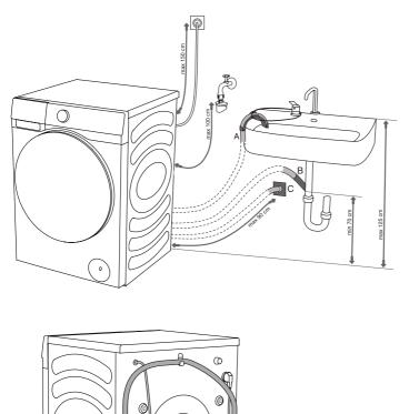
**C** Discharge hose can also be attached to a wall drain with a trap; such trap should be properly installed to allow cleaning.
