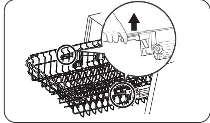
1. To raise the basket to the upper position, lift the basket until both sides are at the same height. The basket will secure into place.
