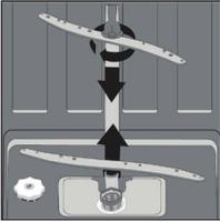
It is essential that you clean the spray arms on a regular basis. In the longer term, waste can block the nozzles and the bearings in the spray arms. Clean the spray arms as follows:
