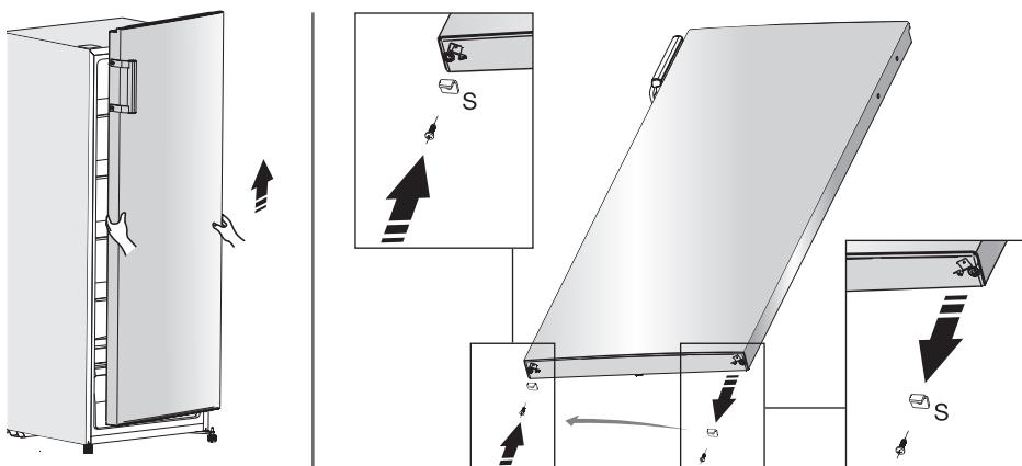
5. Loosen the adjustable feet and the lower hinge and attach them on the other side.
