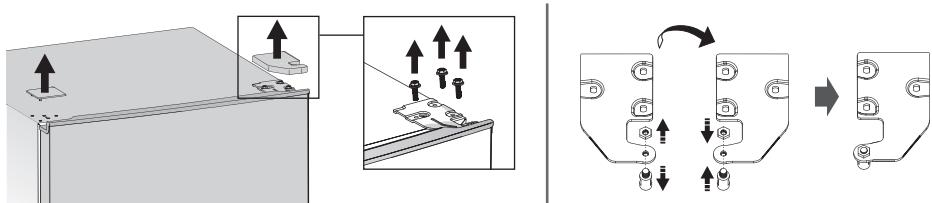
3. Carefully lift the door from the lower hinge and place it on a padded surface to prevent scratching.
