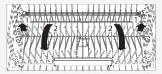
Forward mount for plate support Used for plates with a diameter greater than 25 cm.
