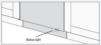
The status light at the bottom on the dishwasher provides information by means of 3 different colours.
