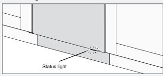
The status light at the bottom on the dishwasher provides information by means of 3 different colours.
