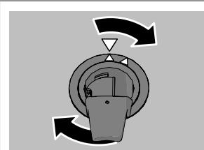
Dishwashing results may be affected if the filters are incorrectly fitted. Note that the dishwasher must not be used without the filters in place!
