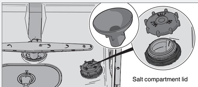
When the salt runs out, unscrew the cap and fill the container with salt. Water is only needed the first time! Wipe clean and tighten. Run a programme to ensure that any salt in the dishwasher is rinsed away.
