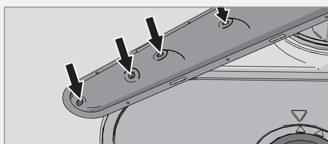
To facilitate cleaning you can remove the spray arms. Remember to fit them firmly back into place afterwards.
