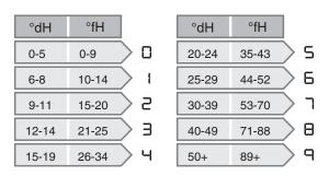
Do not forget to put salt in the salt compartment after you have set the water softener to 1 - 9.
