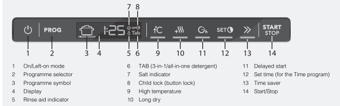
The panel is fitted with touch buttons with audible feedback (see the chapter Settings).
