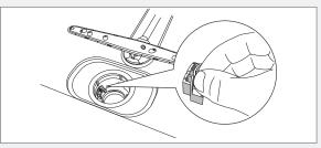
4 By inserting your finger into the hole you can turn the pump blade to release anything blocking it.
