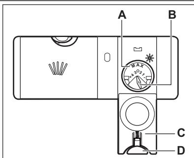
1. Press the release button (**D**) to open the lid (**C**).
