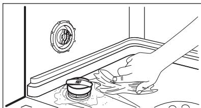
1. Turn the cap counterclockwise and open the salt container.
