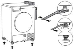
Place the dryer so that it is stable. Use a spirit level to level the dryer in longitudinal and traverse direction by rotating the adjustable feet using a No. 22 spanner (max. 15 mm). Then, firmly tighten the jam nuts (counter nuts) by rotating them towards the appliance bottom using a No. 17 spanner  $\mathbf{1}$ .
