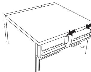
3. Secure the anti-tilt device using the screws as shown in the picture.
