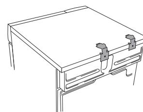
4. Attach the plastic cups for fixing the tumble dryer's front feet to the washing machine's top cover. This is essential, as only when the tumble dryer's feet are resting in the plastic cups can you be sure that the dryer is correctly positioned on the washing machine.
