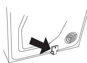
2. Undo the two screws indicated on the back of the washing machine.
