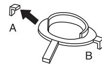
5. Fit the plastic cups so that the "tags" marked with arrows are against the front edge or side edge of the cover and press them firmly onto the cover. Then break off the remaining tags.
