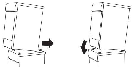
7. Lower the tumble dryer's front feet into the plastic cups and adjust the dryer to ensure that it is balanced.
