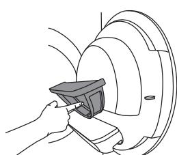
**3** Gently scrape the filter to remove the lint lining (fibres and threads).
