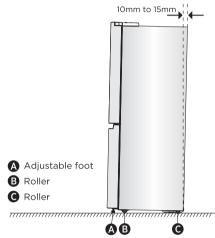
NOTE: Having someone push against the top of the refrigerator takes some weight off the leveling feet. This makes it easier to turn the feet. Rotate the adjustable feet clockwise to raise or raise counter-clockwise to lower your refrigerator. To make sure that the doors close automatically, tilt the top of your refrigerator backward about 10mm to 15mm. If necessary, use a spanner wrench to adjust the feet.
