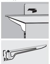
2. To reinstall a shelf, gently slide the shelf back into the refrigerator compartment, and the lower the shelf onto the rail support.
