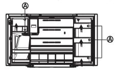
To remove the door baskets (B), take the right side of the baskets out by lifting it at an angle along the guide, and then take the left side out by pulling it from the door.
