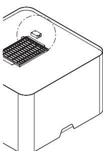
1. Disconnect the cooker hood from the power supply by setting the group fuse in the meter cupboard to '0' or removing the fuse from the fuse holder. If present, the cooker hood can also be disconnected from the power supply with the On / Off switch located at the top of the cooker hood.
