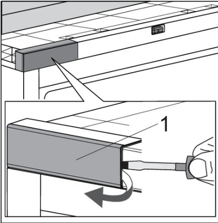
3. Open the appliance door. Carefully remove the upper hinge housing cover (1) with the help of a flat-head screwdriver. Set it aside, as you will need it later on. In case you have changed door opening direction, start in the top right-hand corner.
