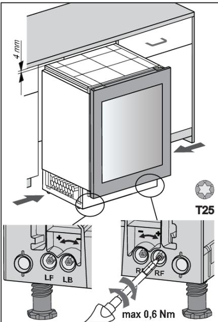
1. Before pushing the appliance into the niche, set the height of the appliance to 4 mm less than the opening. This can be done by turning the adjustable feet: LF - left front, LB - left back, RF - right front, RB - right back.
