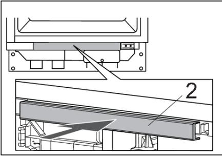
12. Snap the bottom front cover (2) back into its position.
