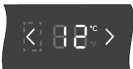
By pressing on the arrow keys, setpoint temperature on display 'T' changes. With every press, setpoint temperature will change 1°C up or down. The setpoint temperature is saved 2 seconds after the last press on temp-up or temp-down key.
