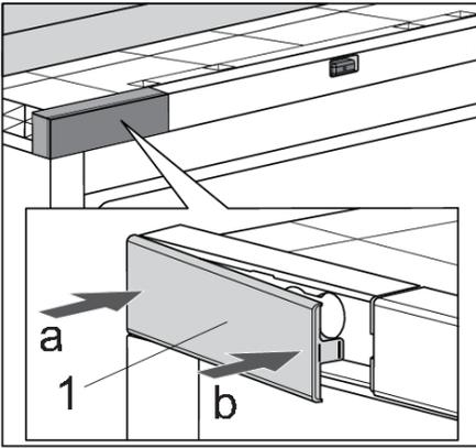
8. Reinstall the upper hinge housing cover (1). First push in the direction of arrow "a" then arrow "b".
