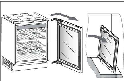
3. Remove the door, complete with the hinges, by moving it in the direction indicated by the arrow. Carefully place the door on the surface prepared for this purpose.
