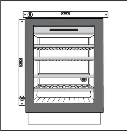
2. The appliance must be aligned horizontally and vertically, otherwise it may deform and it will not be possible to close the door properly.
