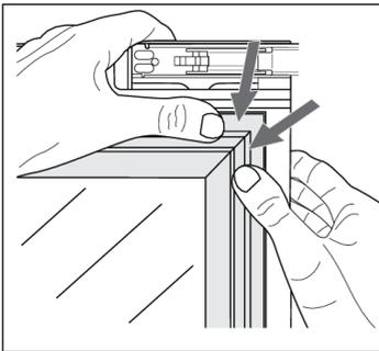
3. Carefully press the gasket back into the groove in the door.
