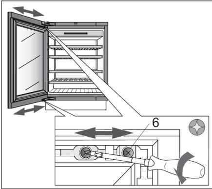
2. Release the screws (6) at the top and bottom. Do not undo them completely! Align the door at the side and tight the screws back.
