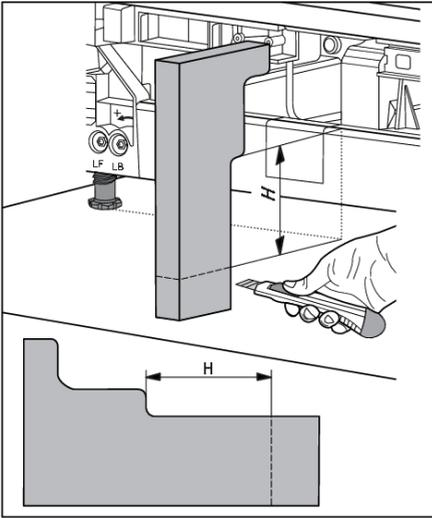
10. Measure dimension "H" on the appliance and then cut the foam airflow divider according to the sketch.
