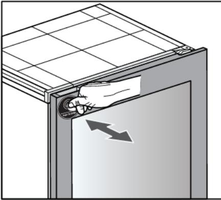
To open the door, push it slightly inwards on the upper left side, then release.
