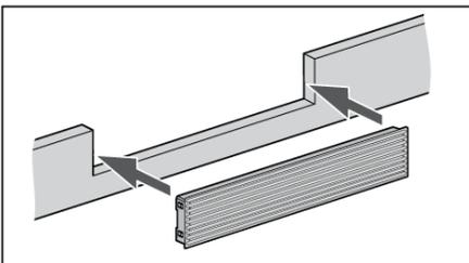
16. Install the ventilation grille into the wooden plinth board.
