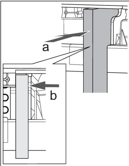
11. Push the foam airflow divider in the direction of arrows "a" and "b".
