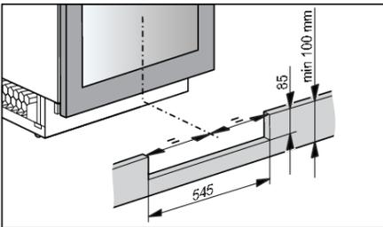
15. Prepare the plinth board. The cut-out in the plinth board for the ventilation grille must be centred with the appliance. This is the only way to ensure correct operation of the appliance.
