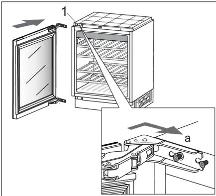
12. Hang the door onto the screws (1) at the top and bottom and slide it in the direction indicated by the arrow (a).
