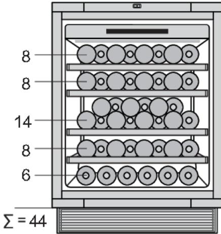
The basic appliance configuration allows storing up to 44 Bordeaux bottles.
