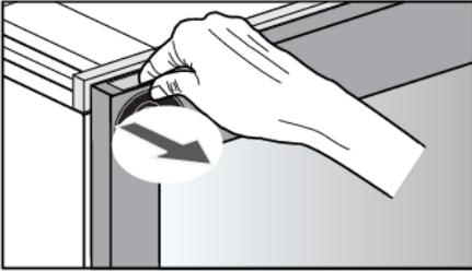
In case of power failure, when push-to-open door mechanism is not operating, hidden handle enables you to open the door.
