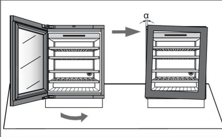
15. If the door is not aligned with the housing (the angle  $\alpha$  is not  $0^\circ$ ),
