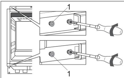
8. Partly attach the screws (1) into the holes at the top and bottom on the left side of the housing.
