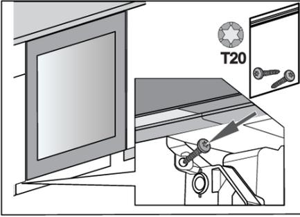
7. Attach the appliance to the adjacent kitchen element at the bottom, on the opposite side of the hinge.
