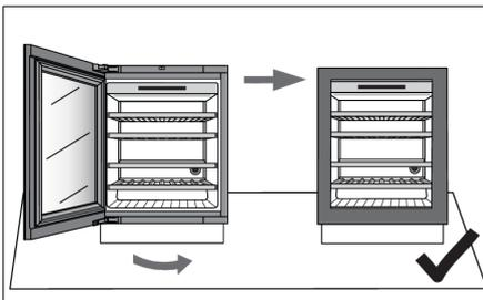
4. The housing side and the edge of the door should be parallel.
