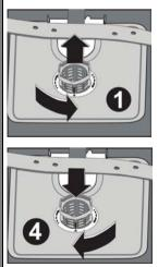
To remove and clean the filter combination, turn it counter clockwise and take it out by lifting upwards.
