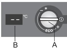
**Switching on:** To switch on: rotate the **A** dial clockwise.
