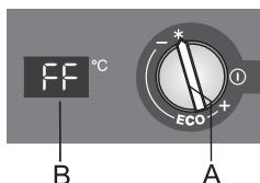
We recommend using this setting before cleaning the appliance or 24 hours before inserting a large amount of food. Activating this function will make sure the food is cooled or frozen faster to retain vitamins, minerals, nutrients, and flavour, and to extend its freshness.
