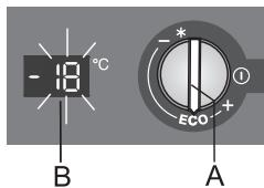
A signal will be given when the temperature in the appliance is too high. The set temperature shown in the display and, if present, the LED lighting will flash.
