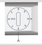
**Turn on**: rotate the thermostat knob clockwise towards position **7**.
