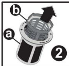
Pull and remove the metal/plastic filter. **3** Then pull the coarse filter out of the micro filter. **2** Rinse it with lots of water under the tap. Refit the metal/plastic filter. Insert the coarse filter into the micro filter in a way that the marks will correspond to one another. Attach micro filter into the metal/plastic filter and turn to the direction of arrow and it is locked when the direction of arrow on micro filter can be seen from across. **4**
