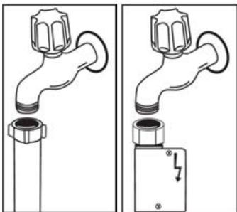
**NOTE:** Aquastop water spout is used in some models. In case of using Aquastop, a dangerous tension exists. Do not cut Aquastop water spout. Do not let it get folded or twisted.
