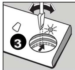
**Warning:** Use only those rinse aid materials which are allowed for use in the machine. As rinse aid residues left as a result of overflowing will create extremely high amounts of foam and thus reduce the washing performance, remove the excess amount of rinse aid by wiping it with a rag.
