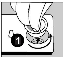
Rinse aid is used to prevent the stay of white water drops, lime stains, white film strip-shaped stains that may form on the dishes, as well as to increase the drying performance. Contrary to the popular beliefs, it is used not only for obtaining shinier dishes but also for obtaining sufficiently dried dishes. For this reason, care should be taken that there is adequate amount of rinse aid in the rinse aid compartment and only polishing material produced for use at dishwashers should be used.
