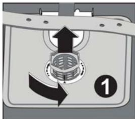
To remove and clean the filter combination, turn it counter clockwise and take it out by lifting upwards. **1**
