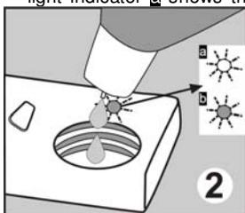
rinse aid. The rinse aid level adjuster can be set to a position between 1 and 6. Factory setting for rinse aid is the position **3**. You need to increase the degree of the adjuster if water stains form on your dishes after a wash, whereas you need to decrease the degree if a blue stain is left when wiped by hand. **3**
