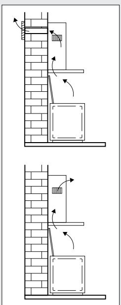
2. Recirculation hood. As a recirculation hood, the grease particles and the smell in the extracted vapours are filtered. The air that has been sucked in is not carried outside but recirculates in the kitchen. In this case you must have a carbon filter fitted.
