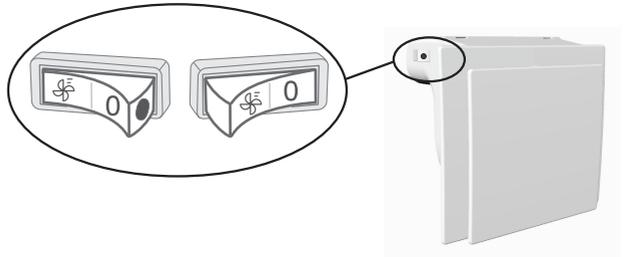
*When the fan and the ionizer are switched on, a red dot will be visible on the switch.*
