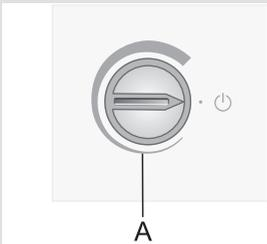
**To switch on:** rotate the **A** dial clockwise.
