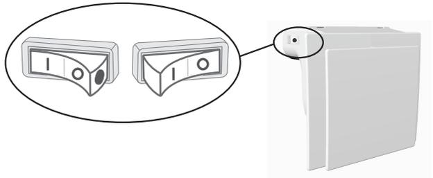
*When the ionizer is switched on, a red dot will be visible on the switch.*
