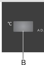
**Conventional appliance** – displays the set temperature of the refrigerator compartment
