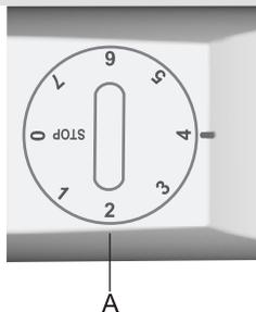
**Turn on:** rotate the thermostat knob clockwise towards position 7.
