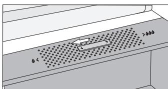
**Slider position to the left:** open vents, lower humidity in the drawer
