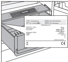
Rating plate can be found in the appliance interior (see figure). It indicates data on voltage, gross and net volume, type and amount of refrigerant, and information on the climate classes.
