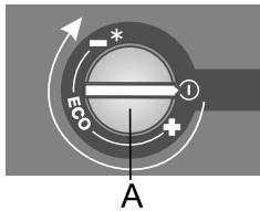
**Switching on:** Rotate the **A** dial clockwise.
