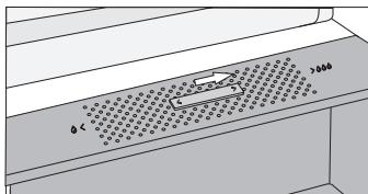
**Slider position to the right:** closed vents, higher humidity in the drawer
