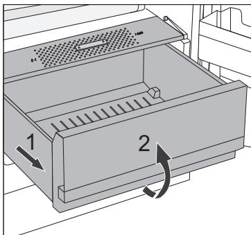
To remove a drawer, pull out the drawer as far as it will go (1). Then, lift the front part (2) and pull it out completely.
