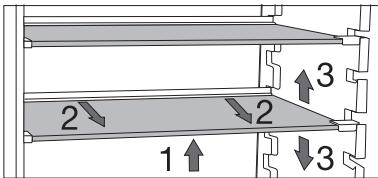
The shelves are made from safety glass. To change the height of a shelf, lift the front of the shelf (1). Take hold of the back and pull the shelf slightly forwards (2). Move the shelf to a higher or lower position (3).
