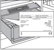
Rating plate can be found in the appliance interior (see figure). It indicates data on voltage, gross and net volume, type and amount of refrigerant, and information on the climate classes.
