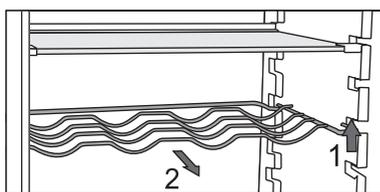
The bottle rack can contain a maximum load of nine 0.75-litre bottles or 13 kilograms of total weight. Also cans can be put on the bottle rack (lengthwise or crosswise). Make sure that the door can close correctly if you have put bottles or cans on the rack. The bottle rack cannot accidentally be pulled out. It can only be pulled out when it is empty. To pull it out, lift it slightly at the front (1) and pull it towards you (2).
