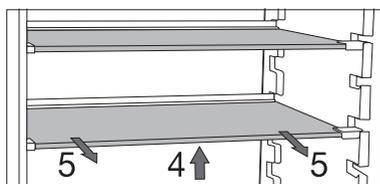
To remove a shelf from the refrigerator, lift the front of the shelf (4). Take hold of the back and pull the shelf out of the appliance (5).
