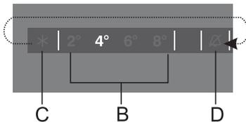
The numbers 2, 4, 6 and 8 indicate the degrees Celsius (°C) in the appliance refrigerator compartment.
