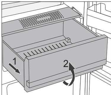
To remove a drawer, pull out the drawer as far as it will go (1). Then, lift the front part (2) and pull it out completely.
