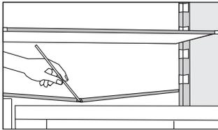
• A gutter and an opening for discharging the water from thawed frost deposits are located underneath the cooling panel that cools the refrigerator interior. The gutter and the opening may not be clogged. Inspect them often and clean if necessary (e.g. with a plastic straw).
