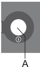
**Switching the appliance on:** Press the **A** key and hold it for 3 seconds.
