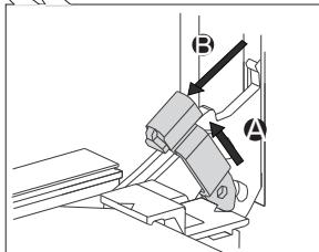
**2** Lift both hinge latches (A) and pull them towards the oven door (B).
