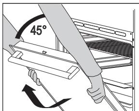
**3** Gently close the door until it reaches a 45° angle. Slightly lift the door and pull it out from both hinge slots on the appliance.
