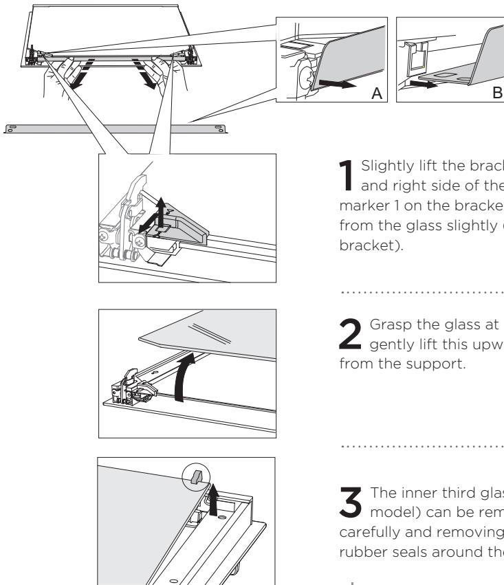
**1** Slightly lift the brackets on the left and right side of the door upwards (to marker 1 on the bracket) and pull this away from the glass slightly (to marker 2 on the bracket).
