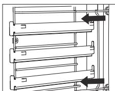
**2** Remove the guides from the holes in the back wall.
