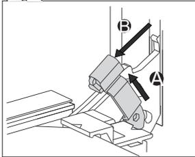
**2** Lift both hinge latches (A) and pull them towards the oven door (B).
