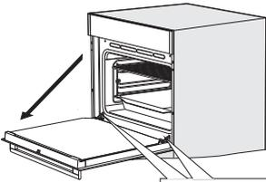
**1** Open the door to the fully open position.
