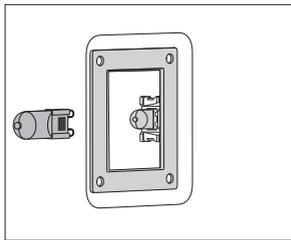
**2** Remove the bulb and install a new one.
