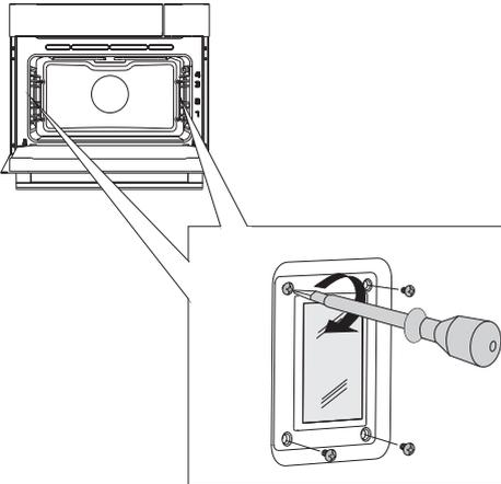
**1** Remove the four screws from the cover panel. Remove the cover panel, the glass and the sealing ring.
