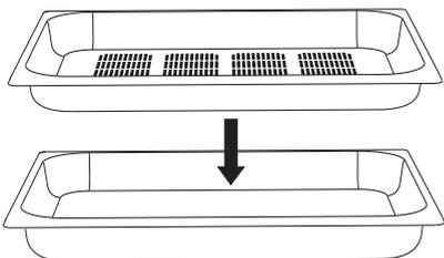
**STEAM SET (INOX)** is used for steam cooking. Place the perforated steam dish in the middle of the oven and the non perforated steam dish one level below the perforated steam dish.
