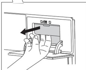
**2** Remove the water tank from the housing by pulling by the recessed part.
