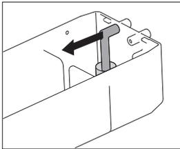
**2** Remove the suction tube with the filter.
