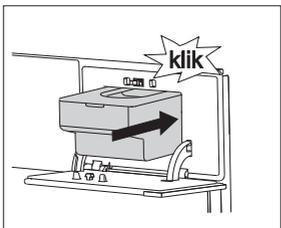
**4** Push the water tank back into the housing to the final position (until you hear a short click). Then, press the tank door to close it.
