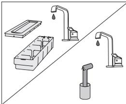
**3** Clean the suction tube and the filter foam under running water. Rinse the filter clean so that there are no visible impurities on it. Thus, you will make sure the appliance operates correctly and preserve the fresh flavour and smell of food.
