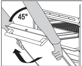
**3** Gently close the door until it reaches a 45° angle. Slightly lift the door and pull it out from both hinge slots on the appliance.
