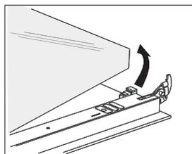
**2** Grasp the glass at the bottom and gently lift this upwards to remove it from the support.
