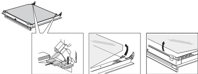
Refit the glass in reverse order. The markings on the oven door and the glass (a semi-circle) need to line up.
