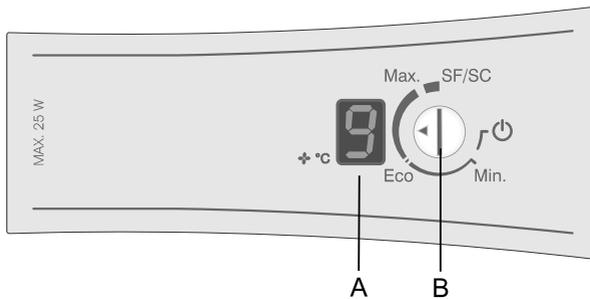
**A Digital temperature display** (certain models only) of the refrigerator indicates actual temperatures during the operation from +1°C to +9°C.
