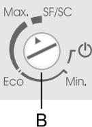
The appliance is switched on by turning the button (B) towards **Max.** and accordingly switched off when the arrow (small triangle) on the button points to the ON/OFF mark
