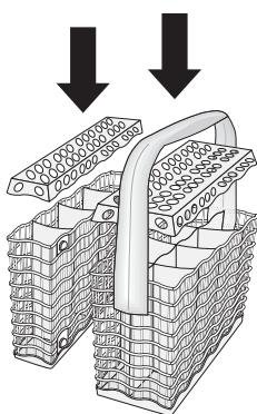
The cutlery basket is in two parts which can be separated to give greater loading flexibility. To separate the two parts, slide them horizontally in opposite directions and pull them apart.
