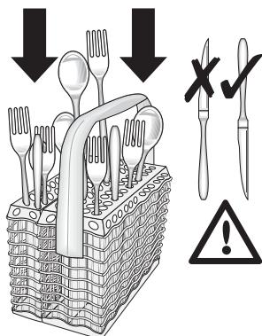
If the handles protrude from the bottom of the basket, obstructing the lower spray arm, load the cutlery with the handles facing upwards. Mix spoons with other cutlery to prevent them from sticking together.
