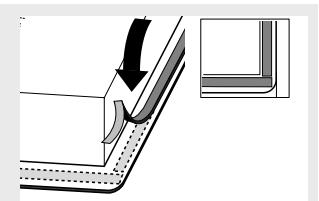
Don't stick the sealing tape around the corner; rather cut four pieces to fit effectively in the corners.
