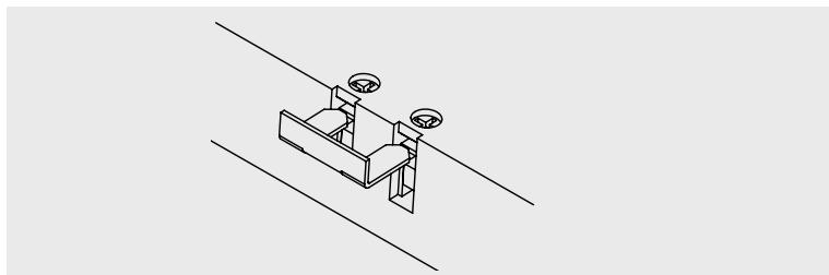
Secure the cable with the strain relief and close the cover.
