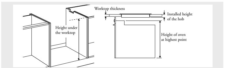
A certain height under the worktop is necessary if the hob is installed above an oven. This height under the worktop depends on the following:
