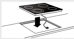
Secure the hob using the fasteners supplied.
