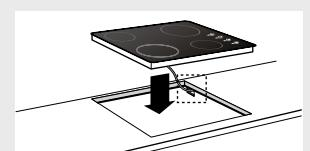
Turn the hob over and allow the appliance to sink into the opening.
