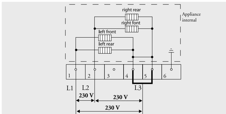
You can use the bridges provided on the connecting block to make the required interconnections as indicated in the preceding illustrations. How to install the bridges is indicated in the junction box cover and in the illustration below. The bridges should not be placed immediately on top of the connecting wires, but between the screw-head and the clamp around the connecting wire.
