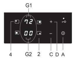
Maximum cooking hob power is limited to 7200 W. This setting can be decreased to 2800 W, 3500 W or 6000 W. The setting can be made within 30 seconds after connecting the cooking hob to the power mains. First, unlock the appliance. Press the cooking zone selector keys 2 and 4 simultaneously. An acoustic signal will be emitted, and the actual maximum power level will be displayed on the displays for the cooking zones G1 and G2. Set the new maximum power level using the (C) and (D) keys.
