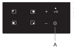
Touch the on/off key (A) and hold it for 1 second to switch off the hob. An acoustic signal will be emitted and all cooking zones will be switched off.
