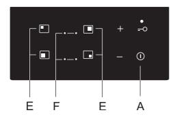
Touch the on/off key (A) and hold it for 1 second to switch on the hob. An acoustic signal will be sounded and the decimal point will light up on all display units.
