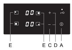
After the hob is switched on (in the next 10 seconds), switch on the desired cooking zone (E). Use the keys C and D to select the desired setting for the activated cooking zone. If you first touch the C key, the power level will be set to "9". If you first touch the D key, the power level will be set to "1".
