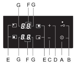
To switch off a cooking zone (E), use the relevant (C) key to set the power level to "O". To quickly switch off the cooking zone, touch the relevant (C) and (D) keys simultaneously. You will hear a short beep, and "O" will be displayed on the display unit.
