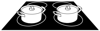
Fig. 6: Zones positioned adjacent to one another can be simultaneously set to level 12.
