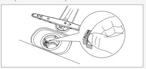
4 By inserting your finger into the hole you can turn the pump blade to release anything blocking it.
