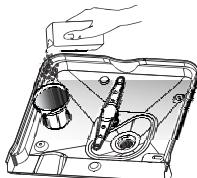
This machine is equipped with a water softener. To use the water softener, fill the dishwasher with salt.
