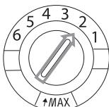
The rinse agent reservoir has 6 settings. To begin with, set the reservoir to setting 2. If this still causes spotting on the dishes and the dishes do not dry well, you can increase the amount of rinse agent added by turning the selector knob on the reservoir to setting 3. If there is still no improvement, turn the selector knob to a higher setting. Repeat this action until the dishes are streak-free when they emerge from the dishwasher.
