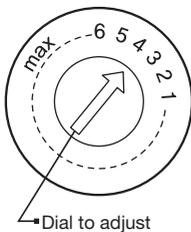
The rinse aid reservoir has 6 settings. Both the recommended setting and the factory setting is "4". If the dishes are not drying properly or are spotted, adjust the dial to the next higher number until your dishes are spot-free. Reduce it if there are sticky whitish stains on your dishes or a bluish film on glassware or knife blades.
