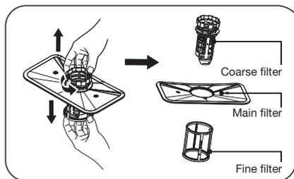
1. Hold the coarse filter and rotate it anticlockwise to unlock the filter. Lift the filter upwards and out of the dishwasher.
