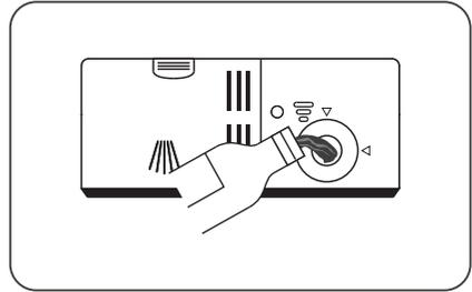
1. To open the dispenser, turn the cap to the "open" (left) arrow and lift it out
