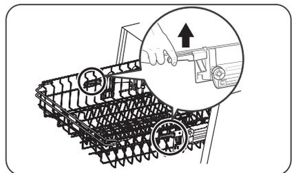
1. To raise the basket to the upper position, lift the basket until both sides are at the same height. The basket will secure into place.
