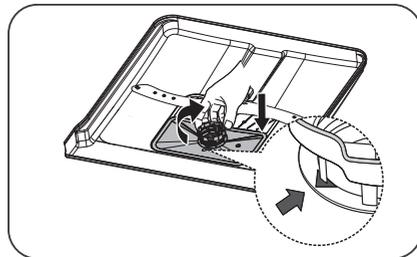
3. Larger food remnants can be cleaned by rinsing the filter under running water. For a more thorough clean, use a soft cleaning brush.
