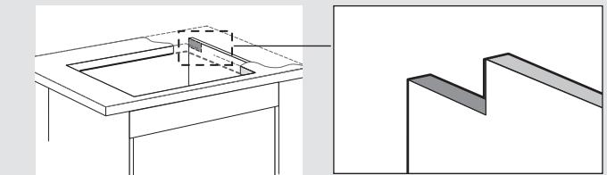
Make a hole in the side of the cupboard for the gas pipe and electricity supply.
