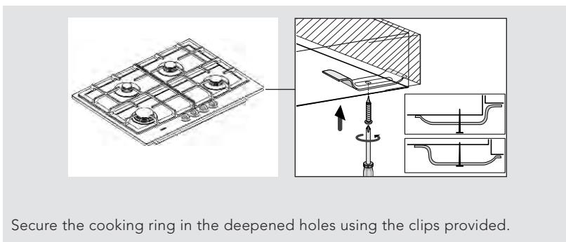
Secure the cooking ring in the deepened holes using the clips provided.
