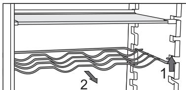
The bottle rack can contain a maximum load of nine 0.75-litre bottles or 13 kilograms of total weight. Also cans can be put on the bottle rack (lengthwise or crosswise). Make sure that the door can close correctly if you have put bottles or cans on the rack. The bottle rack cannot accidentally being pulled out. It can only be pulled out when it is empty. To pull it out, lift it slightly at the front (1) and pull it towards you (2).
