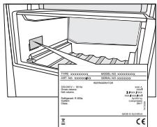
Rating plate can be found in the appliance interior (see figure). It indicates data on voltage, gross and net volume, type and amount of refrigerant, and information on the climate classes.
