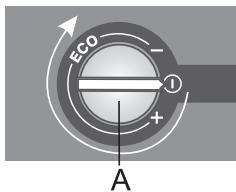
**Switching on:** Rotate the **A** dial clockwise.
