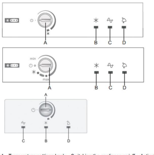
A - Temperature settings knob – Switching the appliance on/off – Activating the super B - Yellow signal light on: Super freeze function is activated
