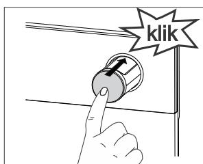
**1** Remove the water tank from the housing by pressing the knob. When you press the knob, the tank jumps out.
