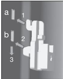
1. Install the hook into hole (a).
