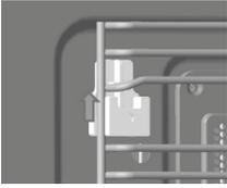
1. Place the bracket against the groove of the hook.
