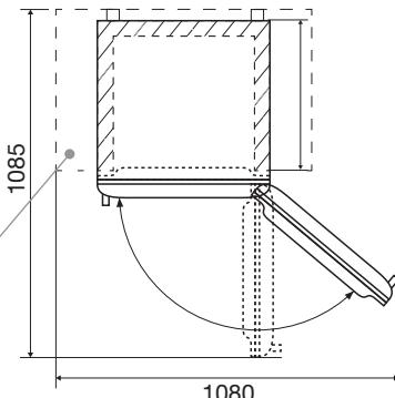
**Provide sufficient space around the appliance to allow for proper ventilation and air flow around the appliance.**
