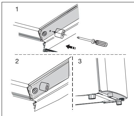
3. Attach the extra foot using a Phillips-head screwdriver (not included).
