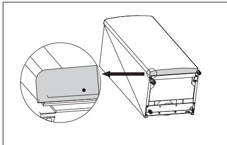
1. Tip the appliance and locate the screw hole at the left side of the bottom.
