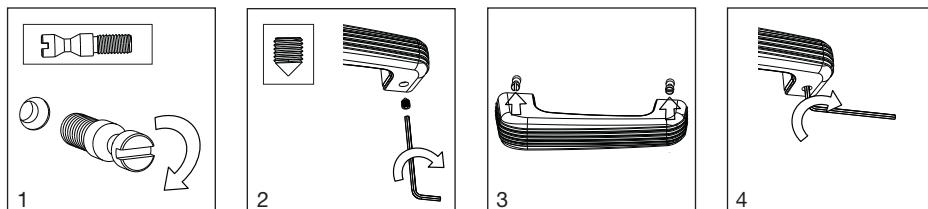
1. Fit the screws in the corresponding holes in the door, using a screwdriver.
