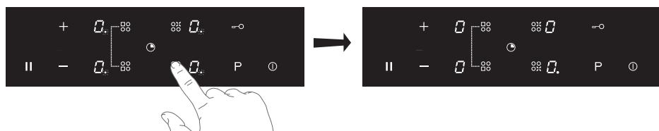
3. Touch the minus (-) or plus (+) key to select a cooking power level. Touch if desired the boost key to start the boost power level.
