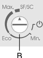
Fast freezing function is activated by turning the button (B) arrow (triangle) to the position SF/SC.
